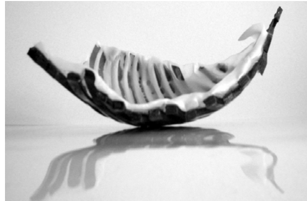
Fig 2 Resin impregnated latex membrane demonstrating curvature induced by pre-stretching.
