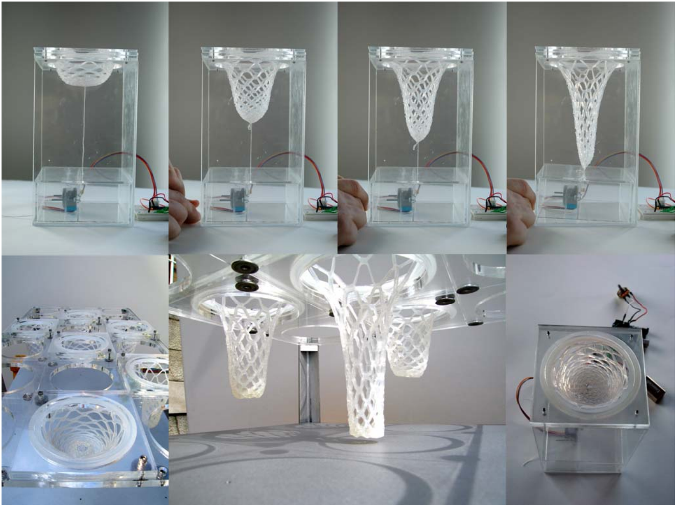
Fig 7 The Homeostat: a 1''=1'-0'' scale model to study the behavior of multiple columns networked together. The control software is tested on this model.
