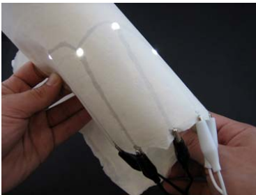
figure 2. Composite combining natural paper and electronic components [2].
